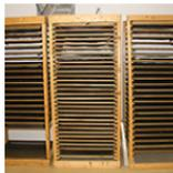
After the wet press, the paper is transferred to a screen shelf on a drying rack. It can take up to two days for the paper to dry. After it has dried, the paper is returned to a second press for the better part of a day. The finished paper is then packed and sent to our studio.
