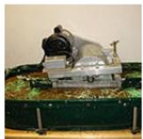
Using a hollander beater, the shredded paper is processed with water into a pulp the consistency of oatmeal. Calcium carbonate is also added to provide an alkaline reserve.
